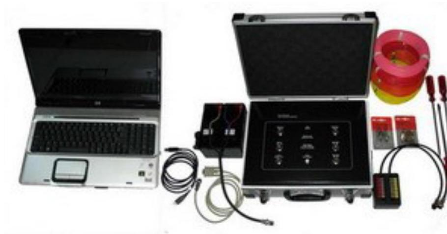
**Gambar 2.** Geolistrik S-Field Automatic Multichannel (Kamur et al., 2020)
